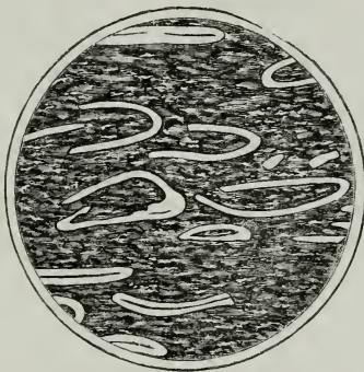
FIG. 69.—Microscopic section of Better Bed coal, Yorkshire. Magnified 25 diameters.
